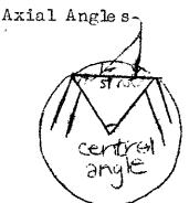
Face Angles are the angles you should find at the tips of your skin panels. Rather than clutter the diagrams by labeling every angle, each angle is only given once. Since the triangle is symmetrical you can easily find the other places it belongs by turning and flipping the triangle:
